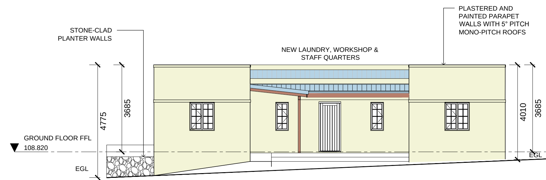
NORTH ELEVATION - NEW OUTBUILDING 1:100
