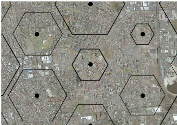
Figure 8 - Coverage decreases due to increase in network users - Cell size decreases.
