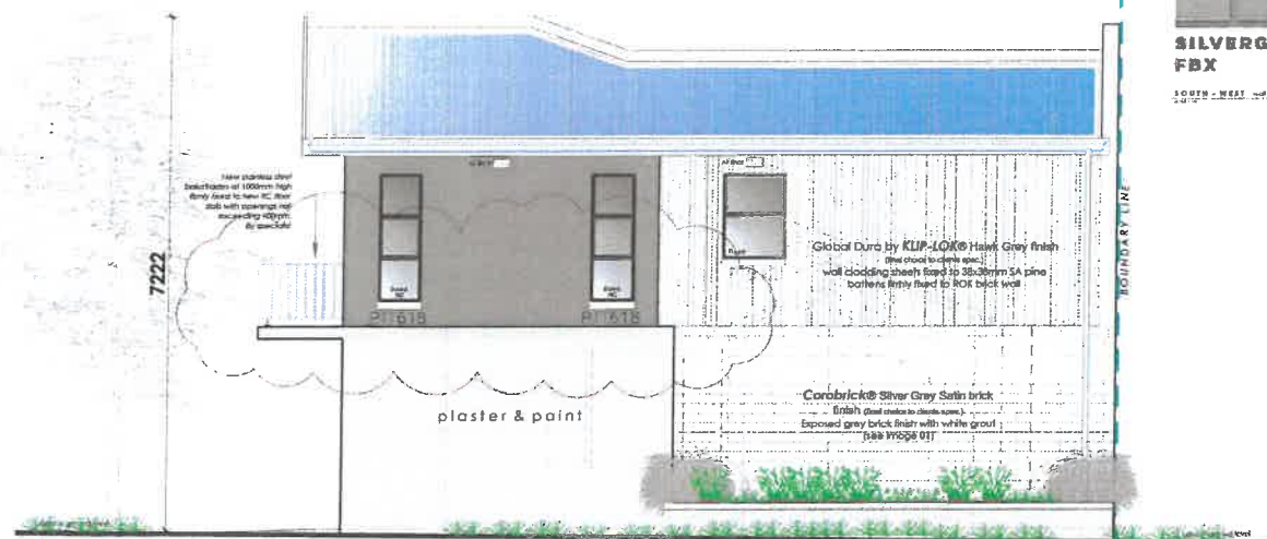
SOUTH - WEST ELEVATION SCALE 1:100
