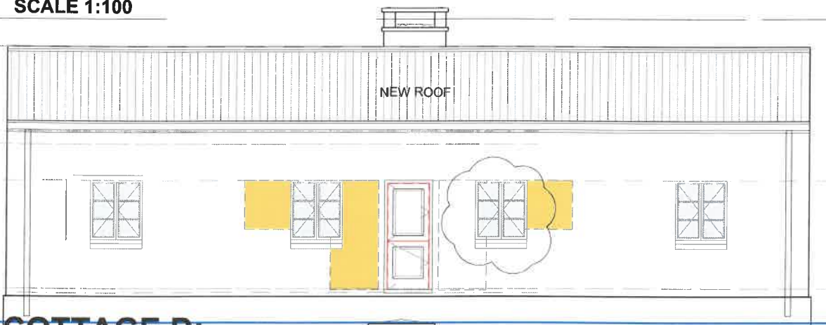
COTTAGE D: NEW BACK ELEVATION SCALE 1:100
