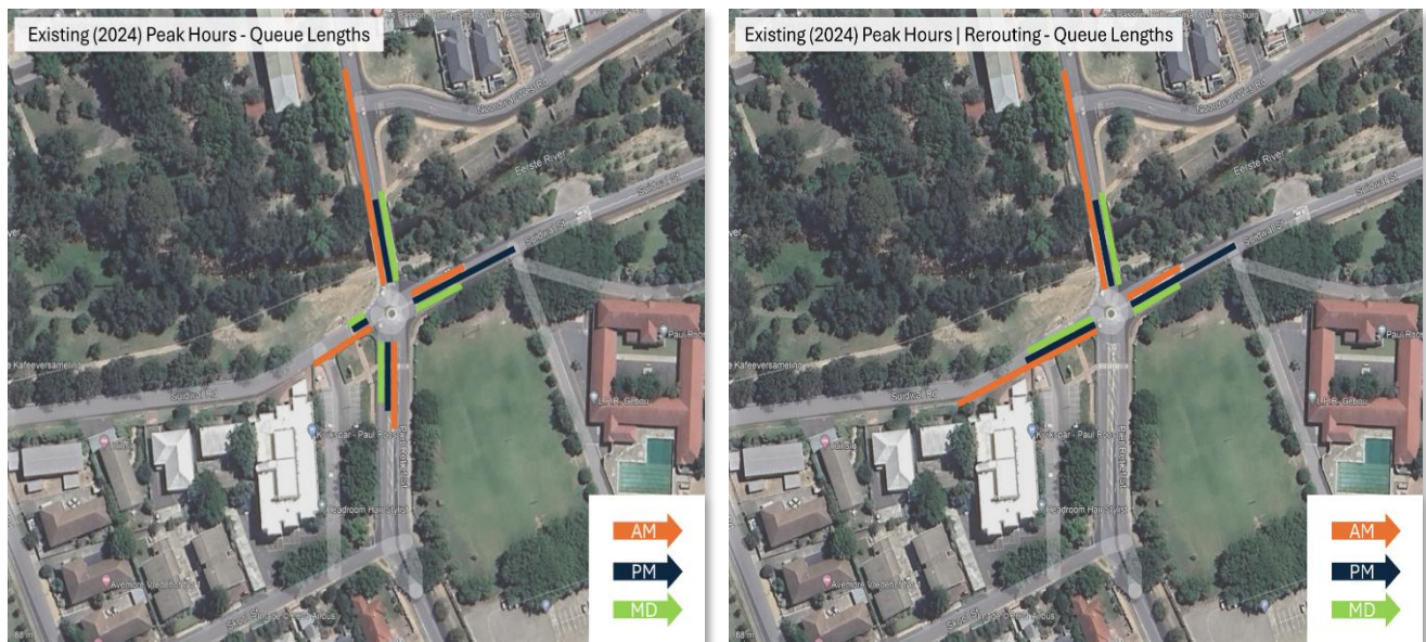
Figure 10: Comparison between existing and rerouted traffic queue lengths (95 th %)
