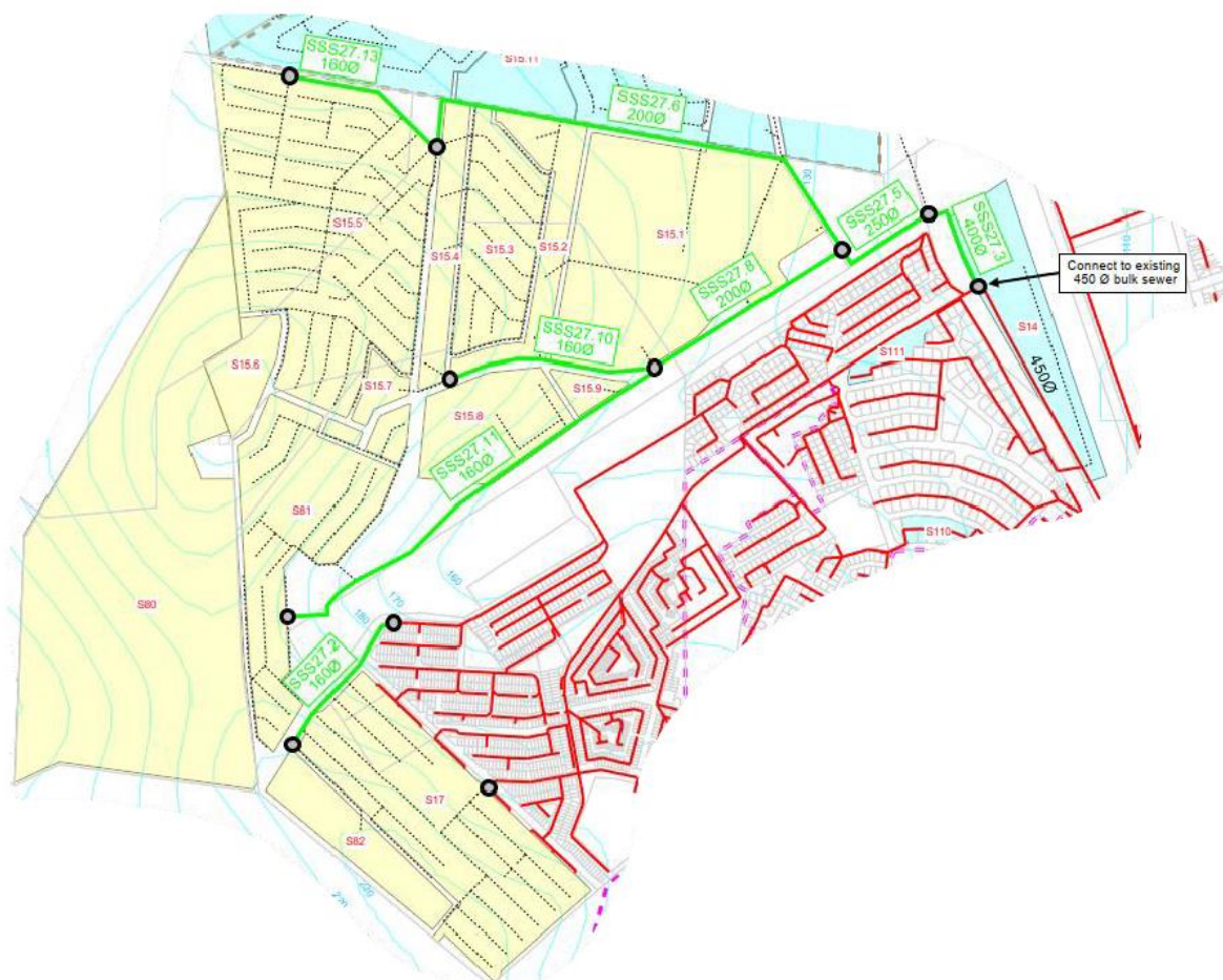
Figure 51 - Bulk sewer distribution upgrades (Municipal Master Plan 2023)
