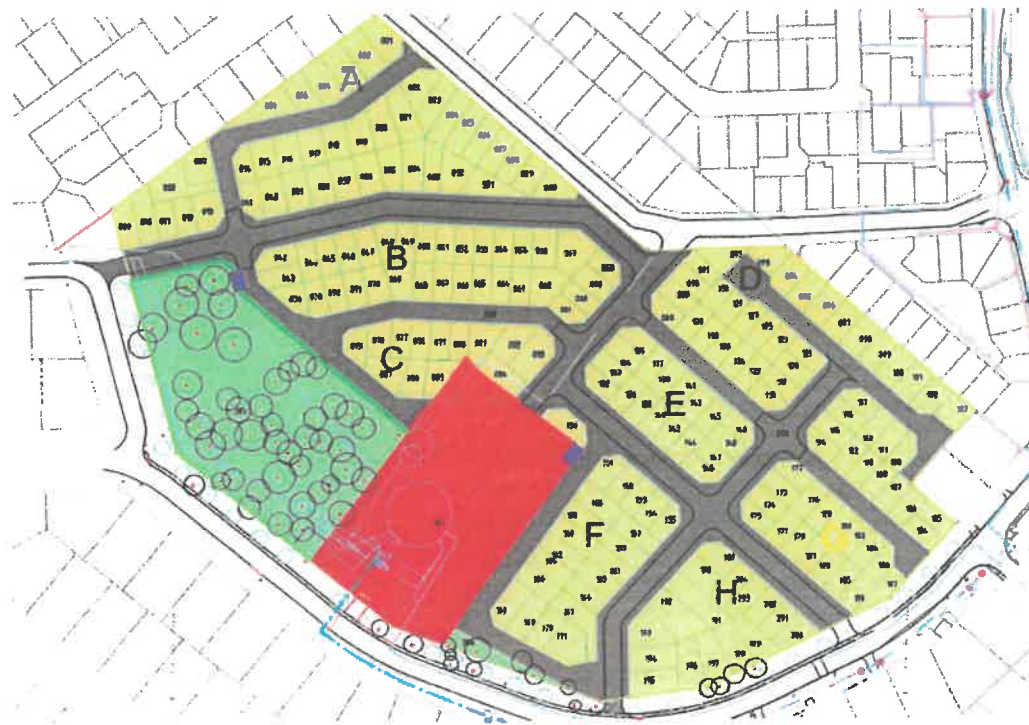
Figure 66 - Indicative positions of electrical substations
