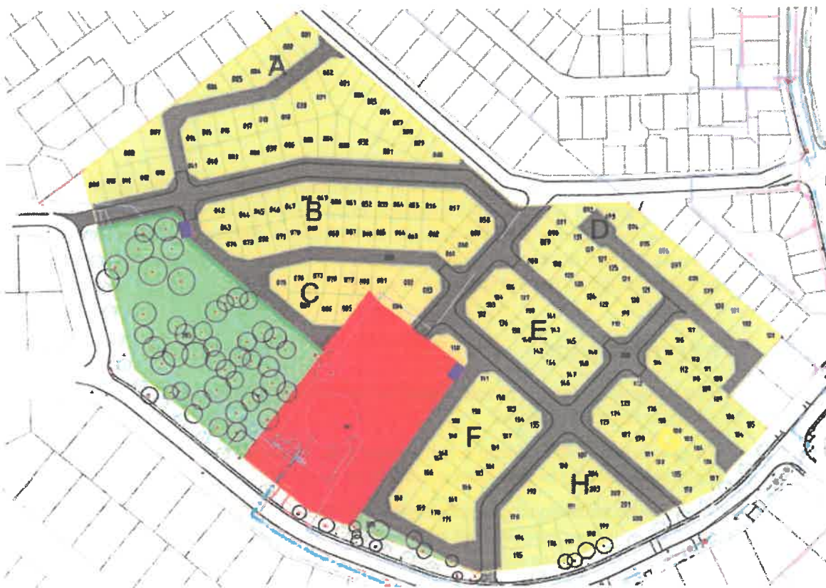
Figure 7: Proposed electrical mini substation positions
