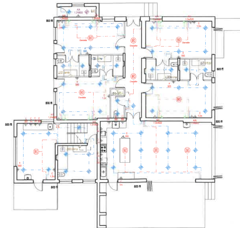
GROUND STOREY ELECTRICAL OUTLAY
