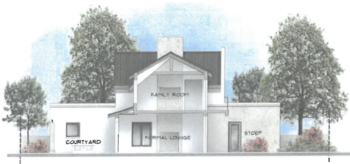
Figure 6: The Core Building with its 40° roof pitch and flat roof abutments.
