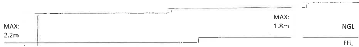
Fig. 2.7.6c. A Diagrammatic Representation of Permissible Shared Boundary Wall Treatment
