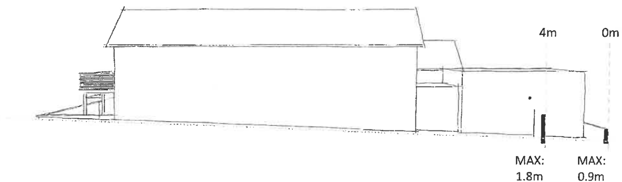
Fig. 2.6.6b. A Diagrammatic Representation of Permissible Location and Height of Street Boundary Walls
