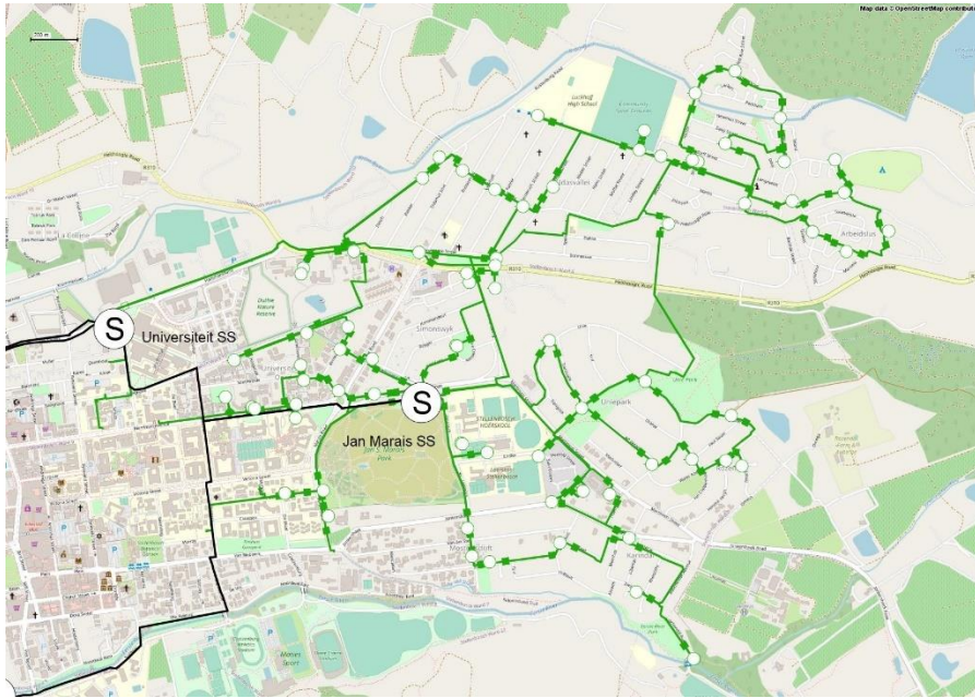
Figure 4-16: Jan Marais substation Electrical Network
