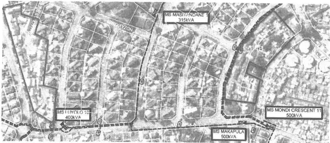
Figure 6 Existing MV Network and Minisubs
