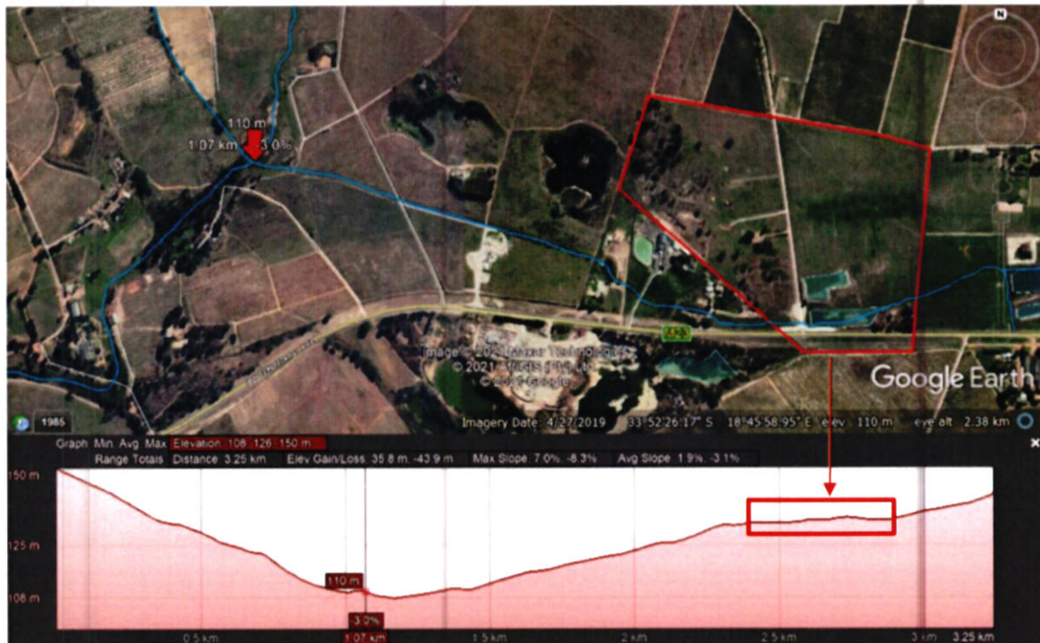
Figure 4. The elevation profile for the tributary of the Bottelary River, shown in Google Earth. The arrow on the image and the corresponding line on the profile indicate the confluence point of the tributary with the river. The red rectangle on the profile indicates the approximate position of the site on the river. The gradient of the river is particularly flat at this point.
