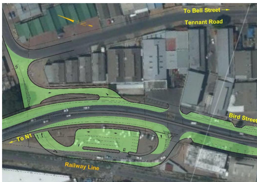
Diagram 1 : Bird Street dualling with Tennant Road link – extract of Conceptual Design
