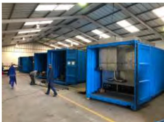
Figure 47: Stellenbosch Containerised WTW being manufactured
