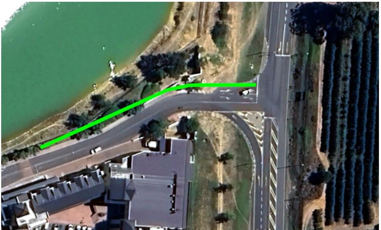
Figure 16: Extension of short lane on Hendrikse Road.
