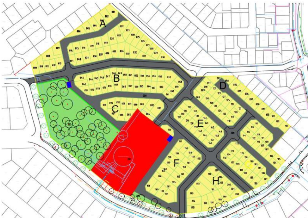
Figure 7: Proposed electrical mini substation positions
