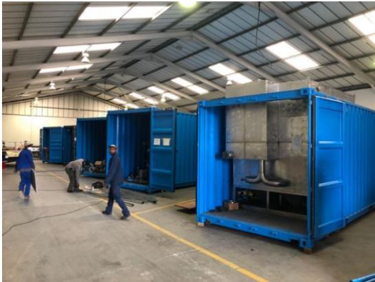
Figure 50: Stellenbosch Containerised WTW being manufactured
