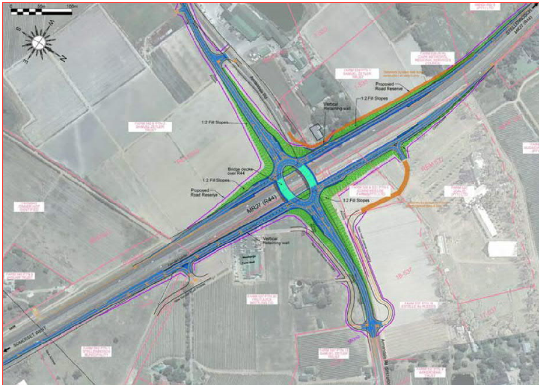
Figure 6-6: R44/Annandale Road grade-separated roundabout with ramp embankments
