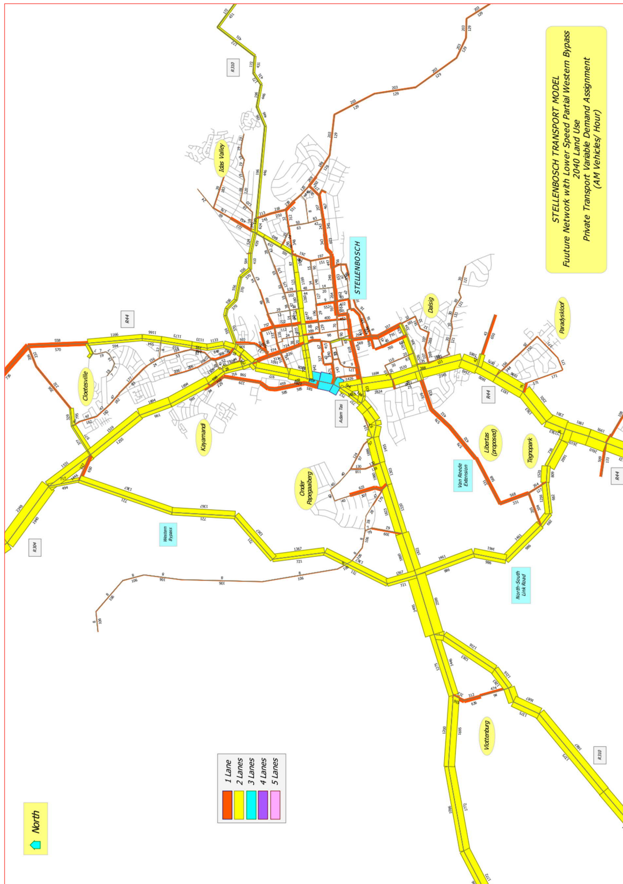
Figure 7-8: Partial Western bypass from grade separated Technopark intersection to R304 (80 km/h) – 2040 Weekday AM peak hour
