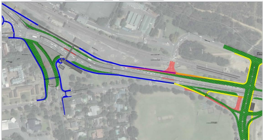
Figure 7-7: Planned upgrade of R310/Alexander Street intersection
