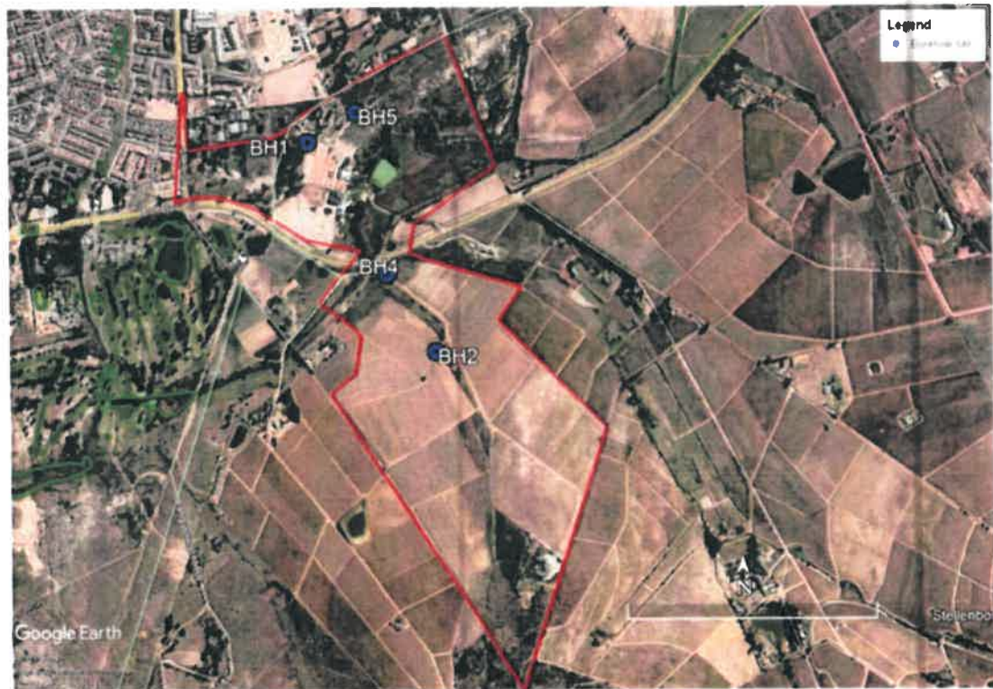
Figure 2.6 Locations of the four boreholes on site (data as supplied by GEOSS)
