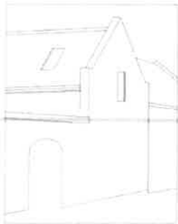
Figure 25: Gable wall with double-pitched roof and parapet
