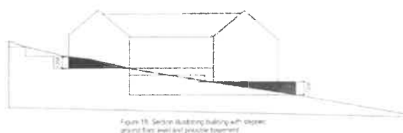
Figure 18: Section through slope illustrating building with stepped ground floor level and possible treatment
