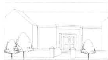
Figure 7: Perspective of Entrance Portico with a flat roof & a width of less than the minimum prescribed width.
