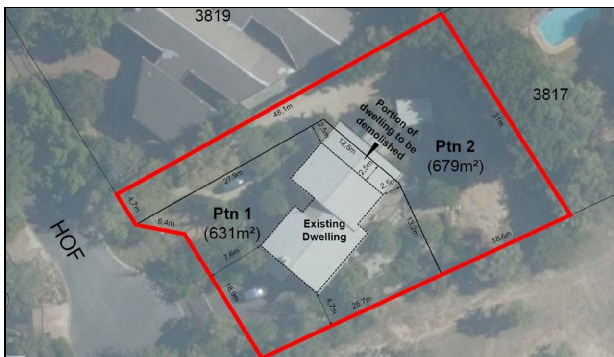
Figure 2: The portion of the existing dwelling that will be demolished
