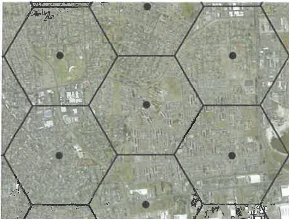
Figure 7- Initial coverage (cell) provided by Telecommunication Base Stations
