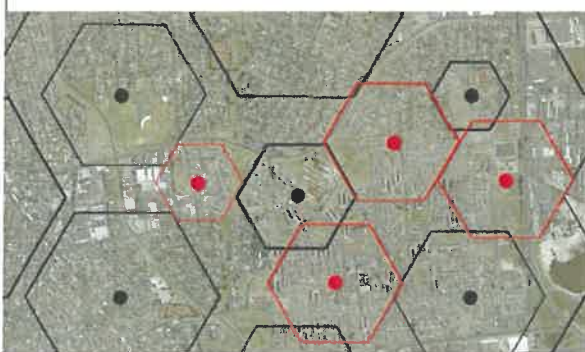
Figure 9 - Additional telecommunication base stations required to fill the gaps
