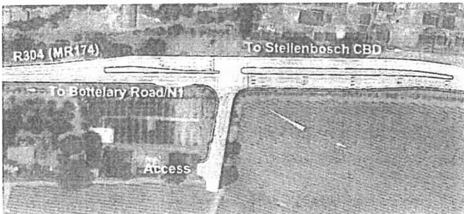
Diagram 1 : Initial R304/Access intersection lane layout (signalised)
