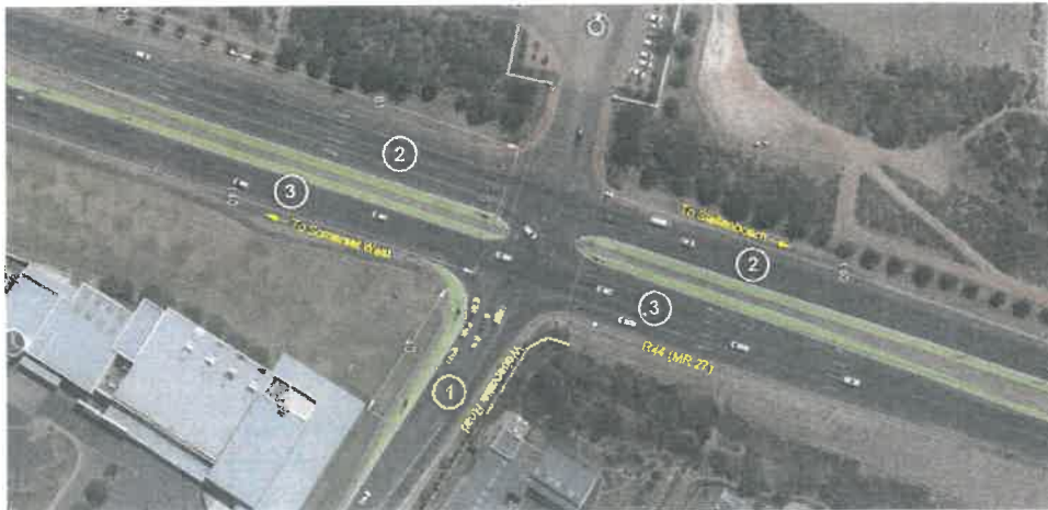
Diagram 1 : Possible upgrade options at R44/Webersvallei Road signalised intersection
