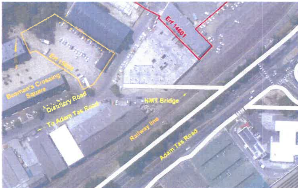
Diagram 1 : Schematic position of NMT bridge over the railway line to directly link the Bosman's Crossing area with the existing NMT along Adam Tas Road
