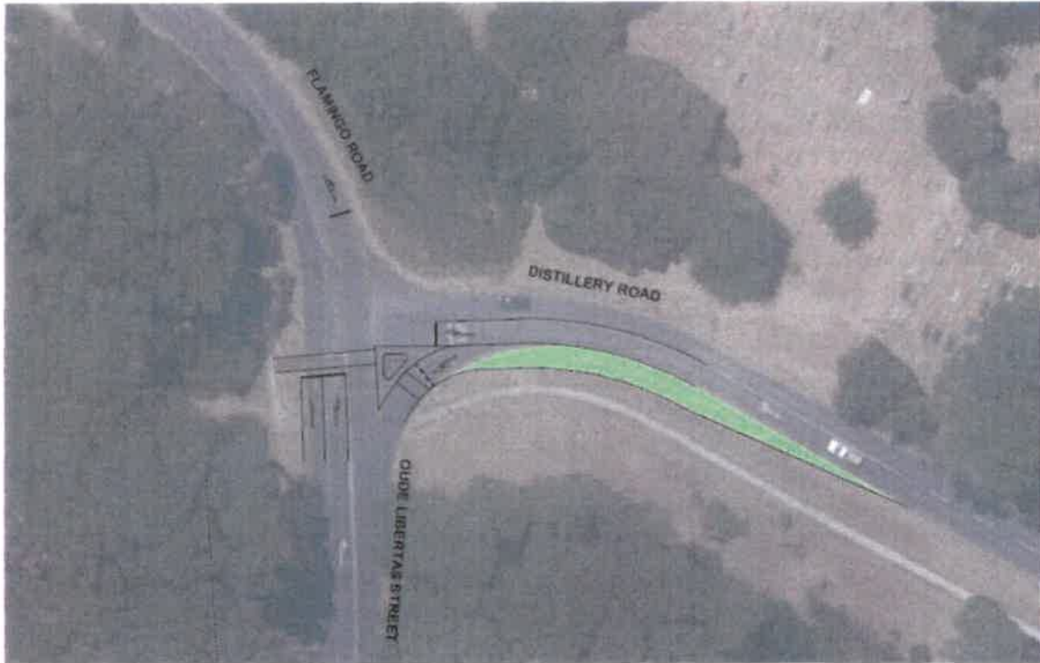
Diagram 2 : Schematic layout of proposed upgrade at Oude Libertas Street/Distillery Road/Flamingo Road intersection
