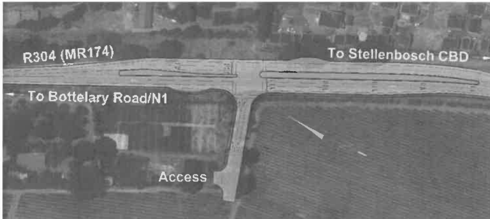
Diagram 2 : Initial R304/Access intersection lane layout (signalised)
