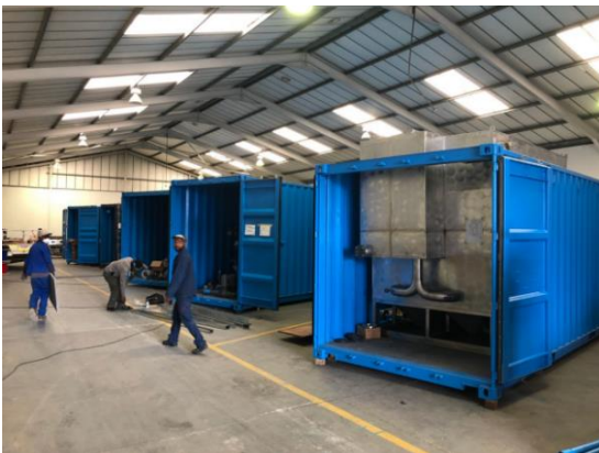
Figure 40: Stellenbosch Containerised WTW being manufactured
