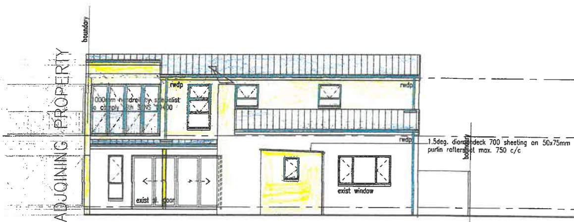
north west elevation 1:100
