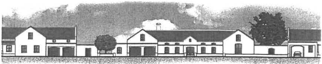
Figure 14: Illustration of linking elements used to connect individual houses and create edge continuity
