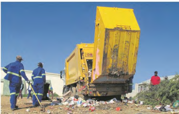
Picture 1: Skips emptied into rear end loaders
