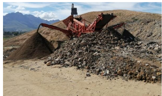
Figure 18: Crushing of builder's rubble done on site
