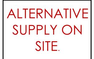
Size 300 x 300 Label to be fitted next to the firemen switch
