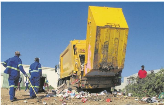
Picture 1: Skips emptied into rear end loaders
