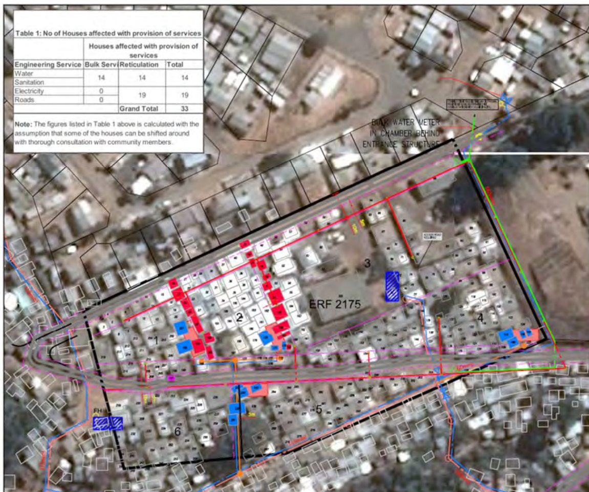
Figure 62 Future electrification approved for 2017/18 financial year
