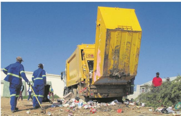
Picture 1: Skips emptied into rear end loaders
