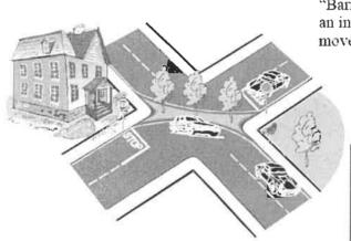
"Barriers placed diagonally across an intersection to prevent through movement."
