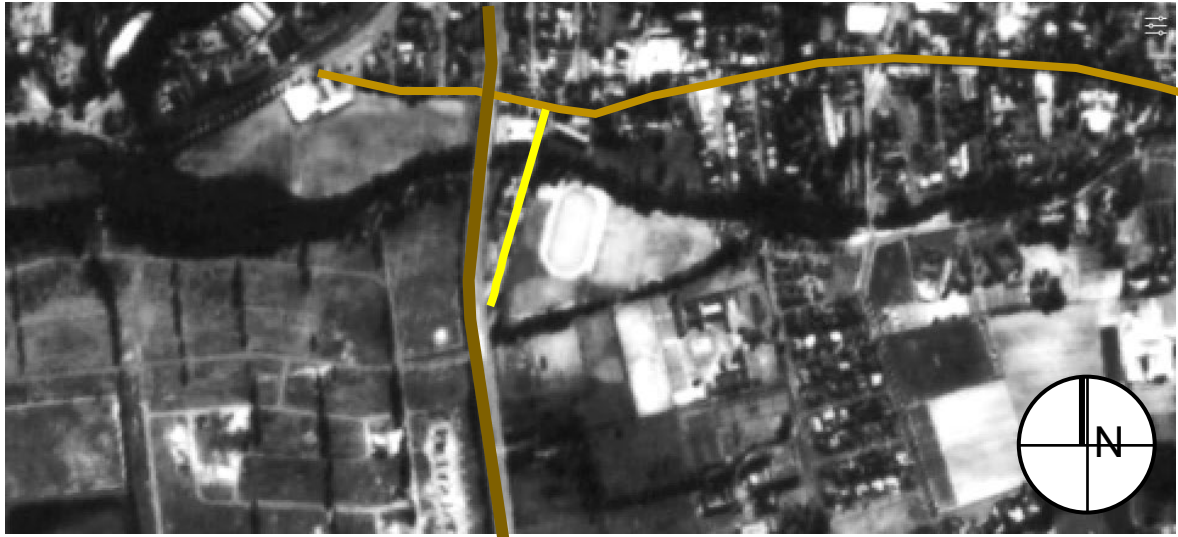
FIGURE 27: 1977: The southern approach into Stellenbosch, now significantly altered with the then recent construction of the R44 (in dark brown) west of the old wagon road (in yellow). The R44 is a north-south through-route across Dorp Street (indicated in lighter brown), bypassing the western end of the town whereas the old wagon road had T-'d into Dorp Street. (SG Historical Aerial Survey Series frame 335_006_06062).
