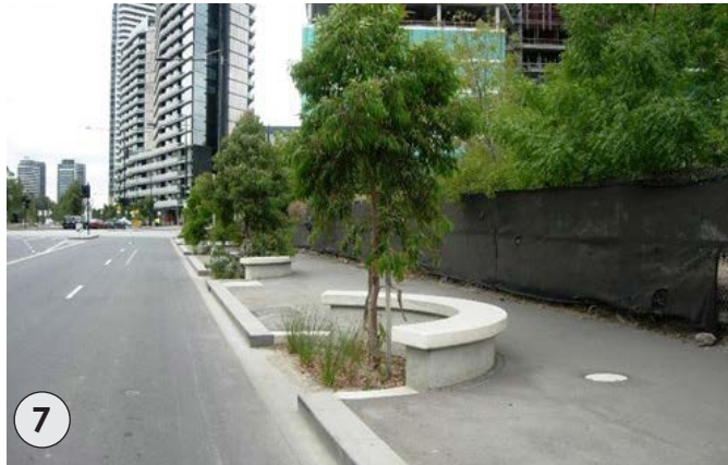
Figure 27. Example of edge activation using tree planting & seating whilst incorporating SUDS design
